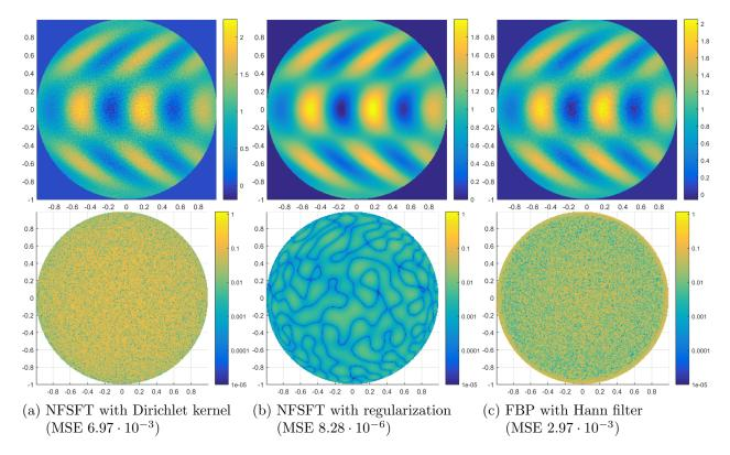
Figure 4: Reconstruction from noisy data with standard deviation 0.01 in the top row and a logarithmic plot of respective errors  $|f - \mathcal{E}f|$  in the bottom row
