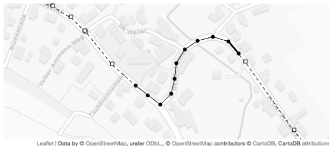
Fig. 2. Illustration of a route on a road map with a resampled mid-section. Square markers represent original nodes from the road map, while circular marker represent nodes resulting from resampling. Dashed edges represent original route segments, whereas solid edges represent resampled ones. In the depicted example, the perceptive field consists of 10 segments, where the target segment is the first segment in the perceptive field (thicker edge).
