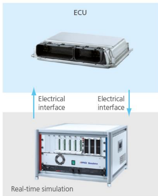
Figure 23 Signal flow in HIL simulation [16].
