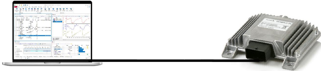
Figure 24 Cost effective HIL platform based on COTS software and hardware.
