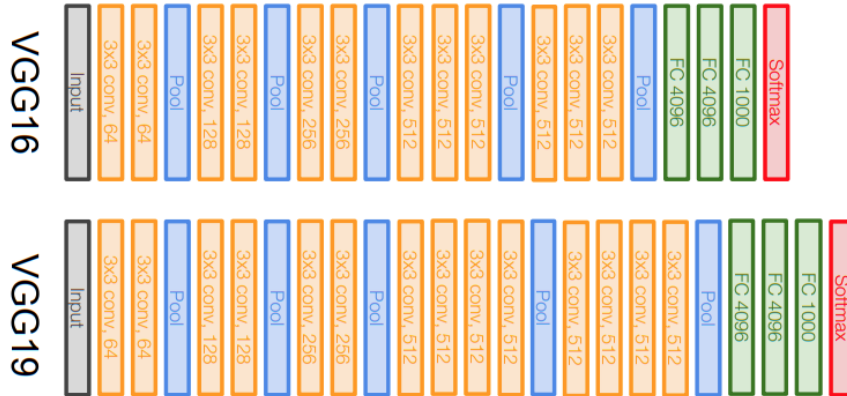
Figure 4.7: The architecture of VGGNet family [24].
